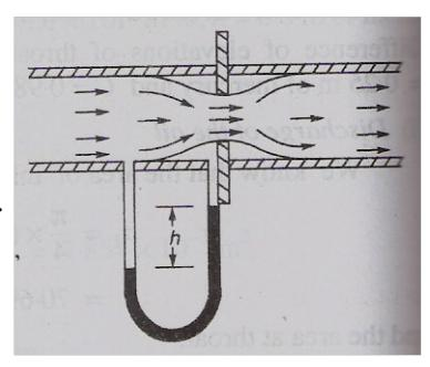
Applying Bernoulli's equation for inlet of pipe and the throat,
